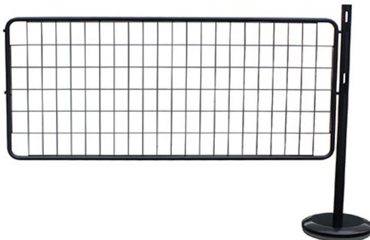
Poteaux hauteur 1000mm. Tube diam 50mm. Grille 1500x650mm. Tube diam 22mm. Maille 65x100mm. Acier.
