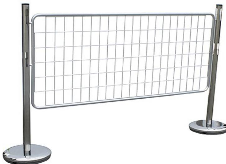
Poteaux hauteur 1000mm, tube diam 50mm. Grille 1600x650mm, tube diam 22mm. Maille 65x100mm. Acier.
